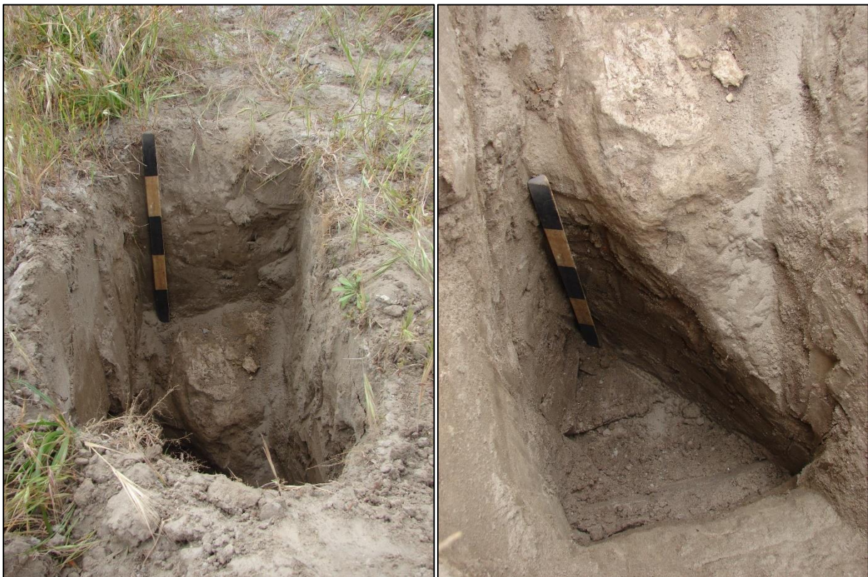
View into Test Hole 25 showing above and below the calcrete boulder. Scale bar = 0.5 m.
