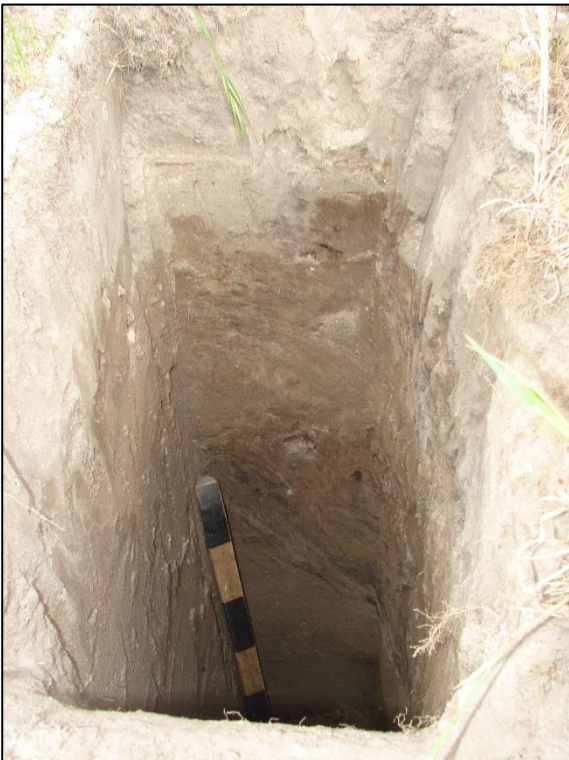
View into Test Hole 14 with the diagonal layers evident. Scale bar = 0.5 m.
